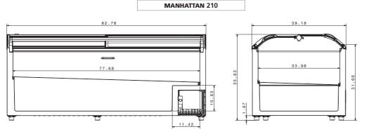
For version AD/U the inner dimensions are reduced due to the necessary use of wire grids along the inside walls.
